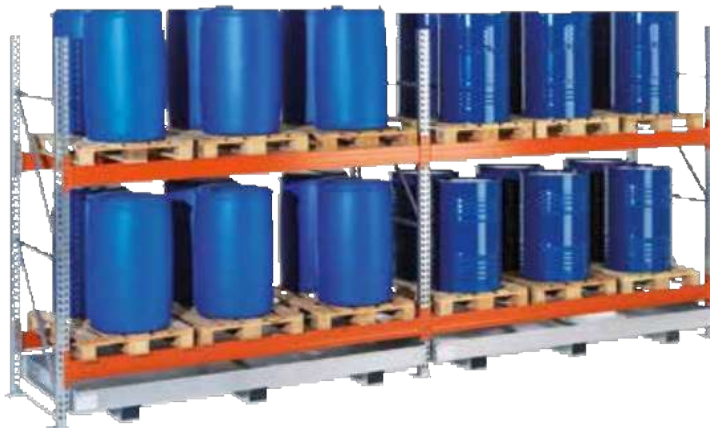
Pallet rack S*2700 mm, 2 levels storage, 12*200 l drum/pallet, tub 360 l b/w galvanised, basic module 124.120.122 incl. add-on module 124.120.123
